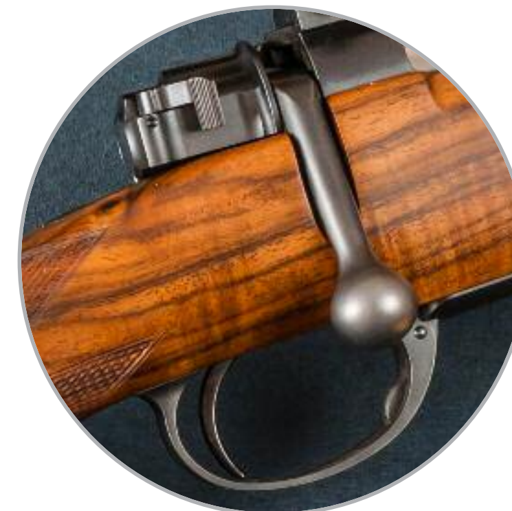
The trigger is nice and crisp, breaking at right around four pounds, with virtually no creep and very little overtravel.
