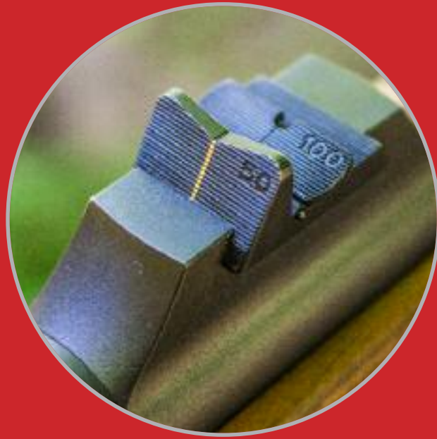
The integral rear sight has a wide "V" for 50-yard shots, and a finer groove for the 100-yard sight.
